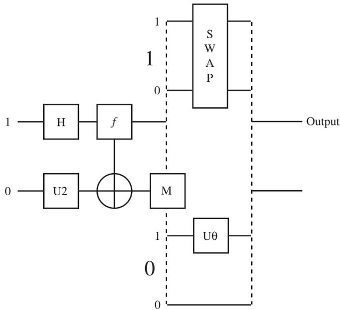
Figure 1: The gate array diagram for an evolved quantum program for the *OR* problem.
