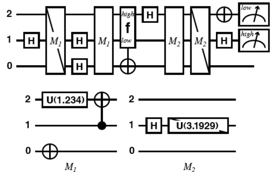
Figure 8.7. A gate array diagram for an evolved version of Grover's database search algorithm for a 4-item database. The full gate array is shown at the top, with  $M_1$  and  $M_2$  standing for the smaller gate arrays shown at the bottom. A diagonal line through a gate symbol indicates that the matrix for the gate is transposed. The "f" gate is the oracle.
